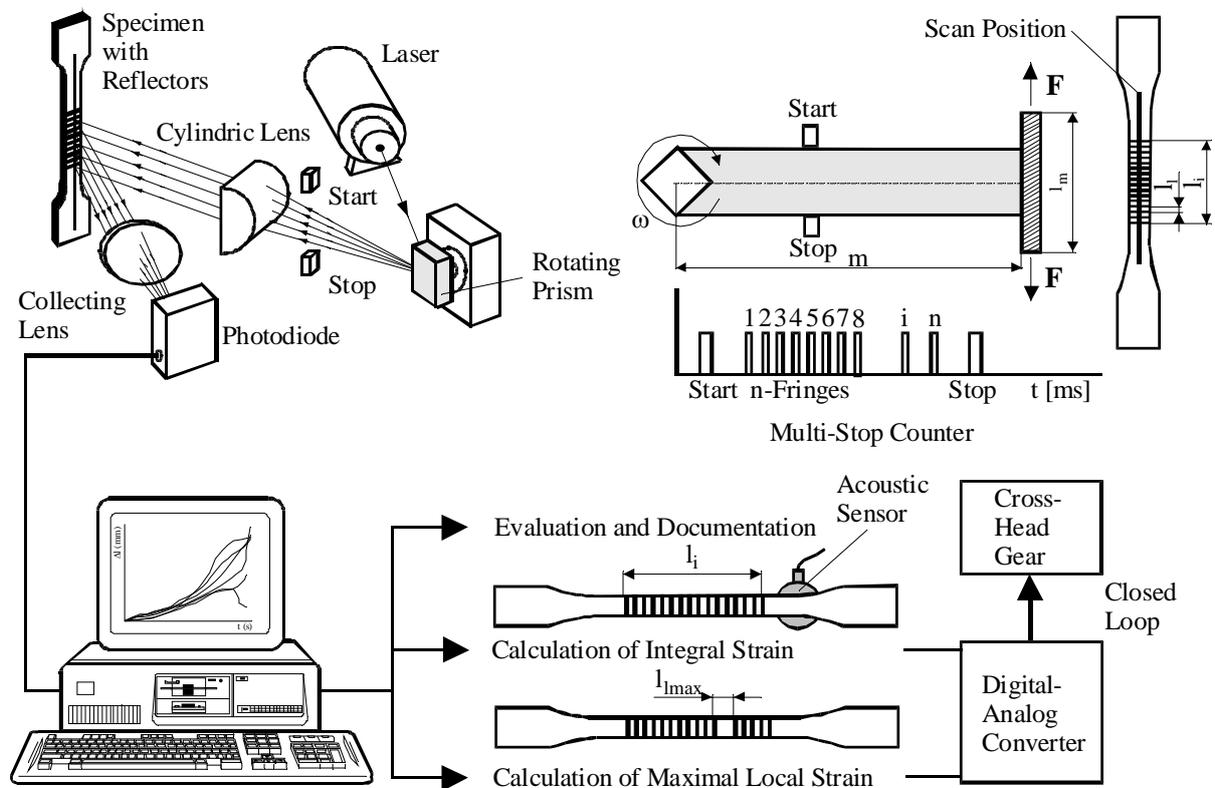
**Figure 1** Principle of local strain measurement and closed-loop experiments by means of the laser extensometer
